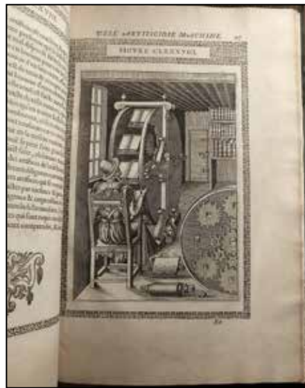
Photo Caption: Drawing from Le diverse et artiose machine del capitano Agostino Ramelli (The Varied and Ingenious Machines) , published in Paris, 1588. The machine shown here is a wheel-operated book-holding device for a scholar who suffers from gout. Rare Books and Special Collections Division, Library of Congress.
